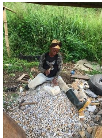
Figure 55: Women breaking stone to make gravel, limited use of PPE, gravel crushing site at Song Nleng
