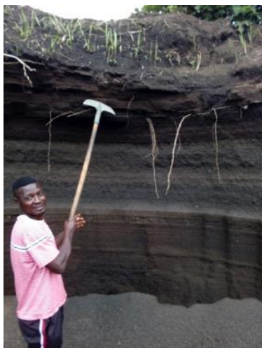
Figure 109: Worker excavating various layers of pozzolan
