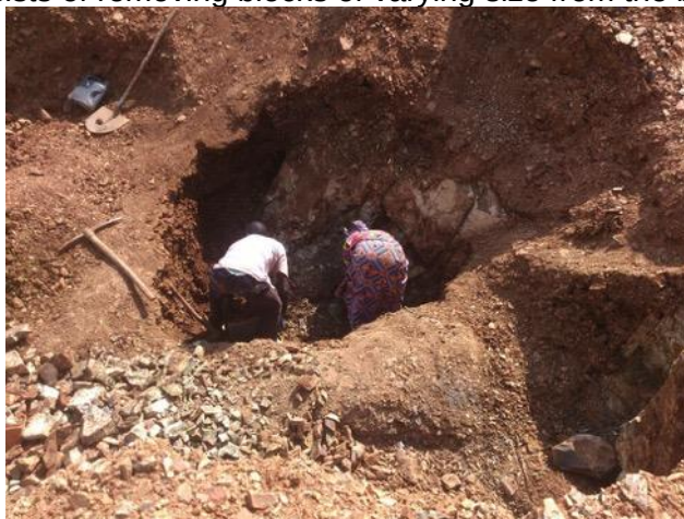
Figure 119: Extraction of rubble from the mother rock
