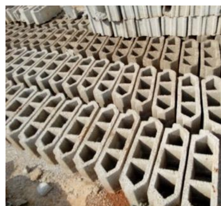
Figure 86: Ourdi used for cement platform, Nkometou
