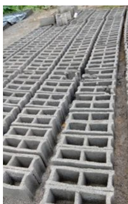
Figure 84: Breeze blocks used for house building, Nkometou
