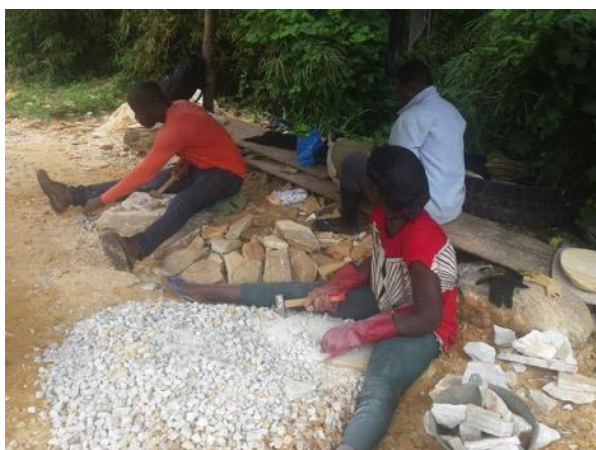
Figure 71: Male and female workers crushing gravel at Missingléo
