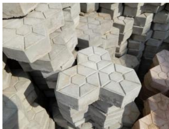
Figure 83: Pavement used for external flooring, Nkometou
