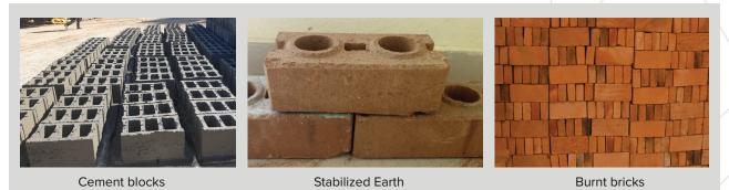
The study found that Stabilized Earth Bricks are one of the lowest-emission material compared to other materials. The only exception is unburnt bricks (mud bricks), which in the case of Yaoundé have the lowest emissions. However, mud bricks are poor quality and are not resistant to extensive rains and floods. In contrast, burnt clay bricks are the highest emitting material-this is due to their large impact on deforestation.
