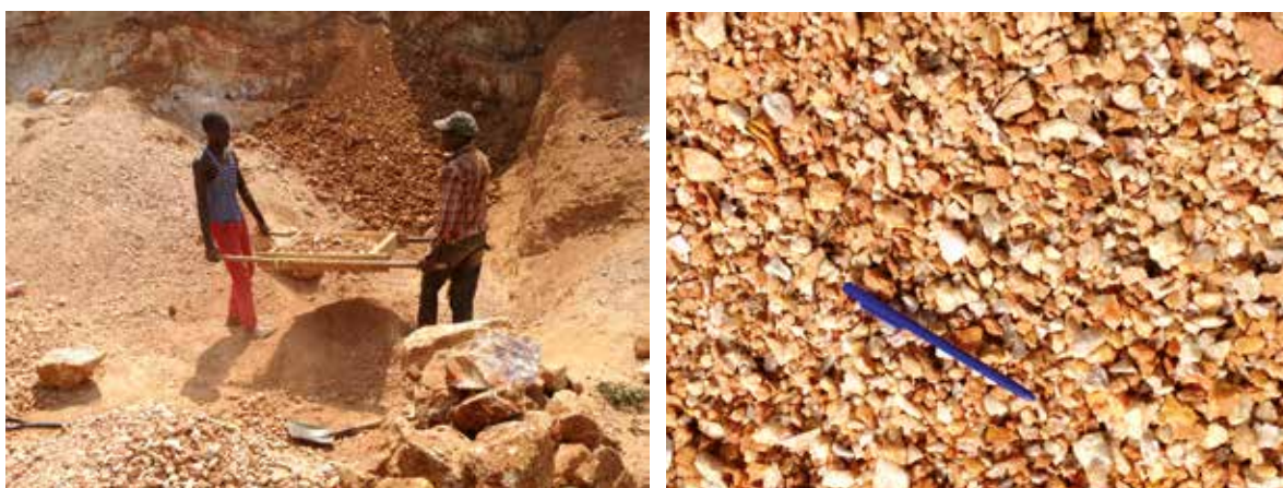
Figure 30: Although sieving is practiced at many sites, the size ranges within most products often do not adhere to national standards for different applications
