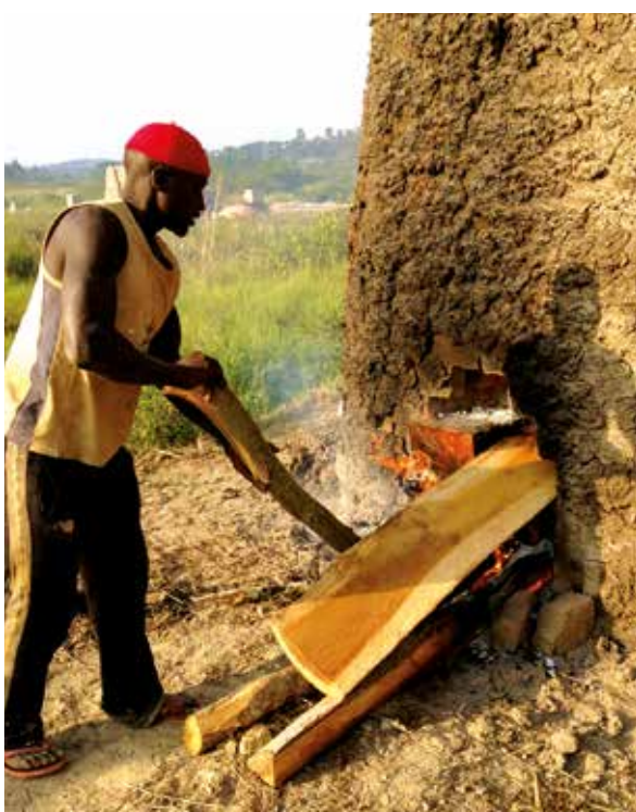
Figure 19: Sun-drying of bricks (top right), loading a kiln with wood (bottom left) and burnt bricks awaiting sale (bottom right). Photo: Levin Sources (2017)
