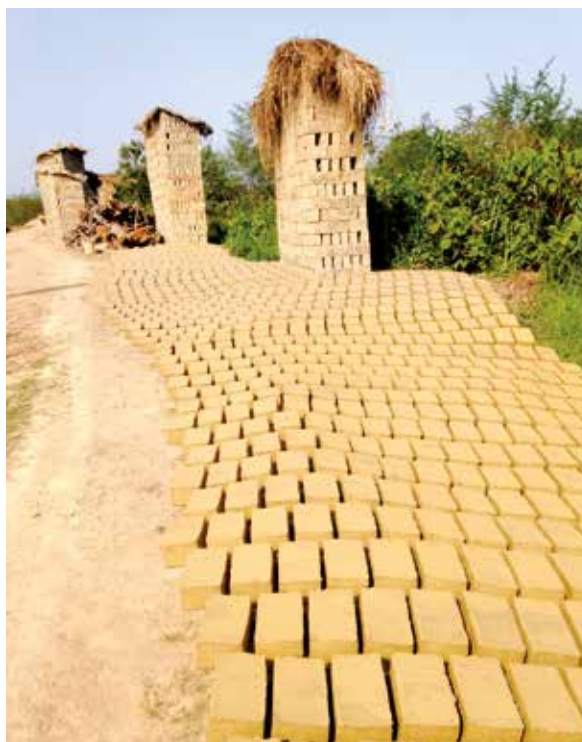
Figure 19: Sun-drying of bricks (top right), loading a kiln with wood (bottom left) and burnt bricks awaiting sale (bottom right). Photo: Levin Sources (2017)
