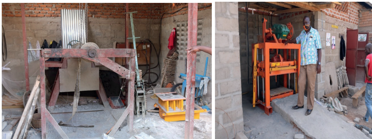
Figure 6: LEFT: A locally fabricated block - making machine at a small-scale factory in Lira City. RIGHT: A Multi-purpose Chinese-made imported block-making machine.
