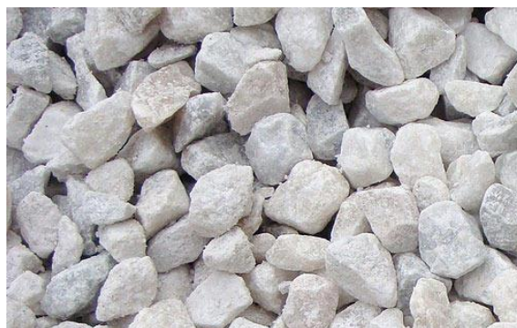
Fig. 20 : Aggregate from crushed marble produced by ASM
