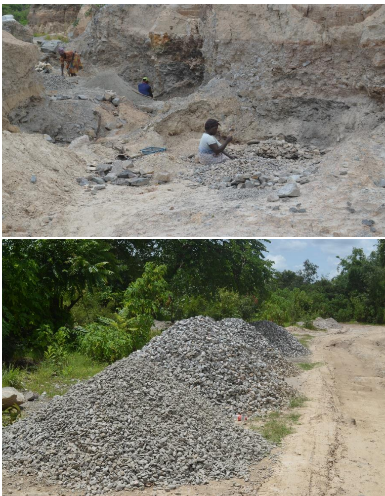
Fig. 7: Aggregate production from a Mine waste dump at Lesa Wamaka Association Site in Kalulushi. Photo credit: Nixon Chisonga.
