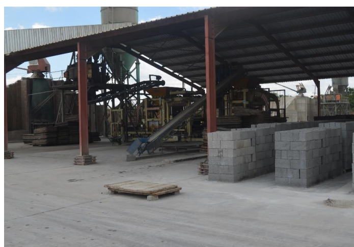
Fig. 8: Concrete block making from aggregate produced at Oriental Quarries Site in Makeni Konga Area, Lusaka, Zambia. Photo credit: Nabita Zaloumis.
