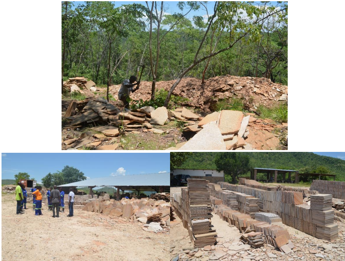
Fig. 12: Field photographs showing the Zambezi Natural Stone Company mine site (top) and plant (bottom) in Siavonga for production of dimension stone (micaceous banded quartzite). Photos courtesy of Nixon Chisonga.
