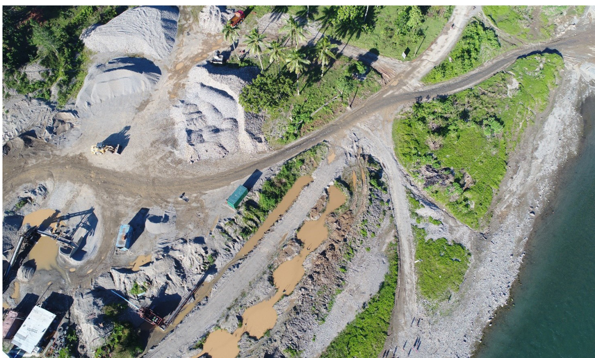
Gravel stockpiled on a river bank in Fiji, exposed to flood risk.
