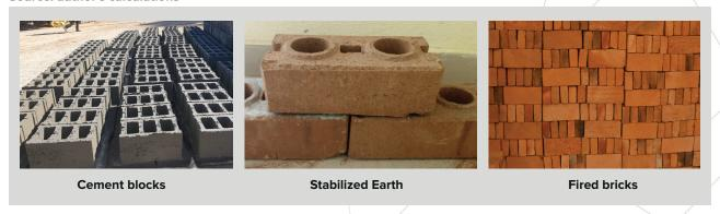
The study found that Stabilized Earth Bricks are one of the lowest-emission material compared to other materials. The only exception is unburnt bricks (mud bricks), which in the case of Yaoundé have the lowest emissions. However, mud bricks are poor quality and are not resistant to extensive rains and floods. In contrast, burnt (fired) clay bricks are the highest emitting material-this is due to their large impact on deforestation.
